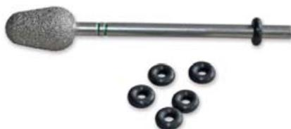
Position the dust protection ring approx. 5 mm from the lower end of the grinder shaft. Push the grinder with the dust protection O ring into the hand piece to the stop.
